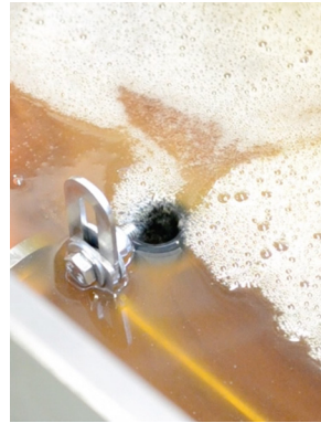
Weir transfer - No levels to set
