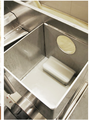
Clean coolant returned to sump
